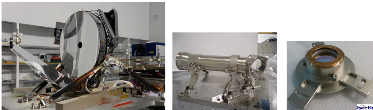
Figure 15: ATLID receiving telescope- Blocking Filter and Entrance filter units.
