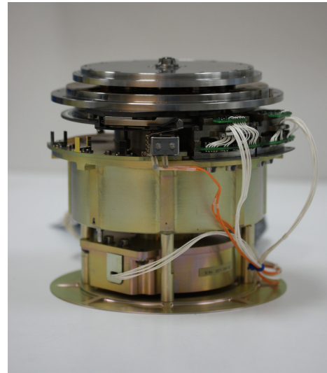
Figure 24. Flight Mechanisms Assembly. The assembly is standing on the radiator and wiring to the chopper mechanism encoder is visible in the bottom section. At the top of image the circuit cards of the calibration mechanism encoder are visible. The discs at top of image interface to calibration and chopper drums.
