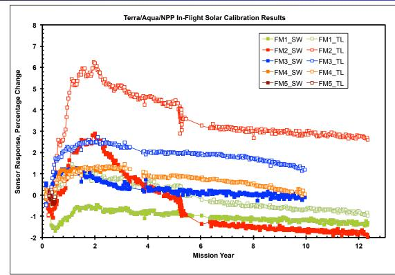
Si02 overcoat on the CERES FM1-FM4 Solar diffusers not applied properly, and continued to oxidize on orbit
